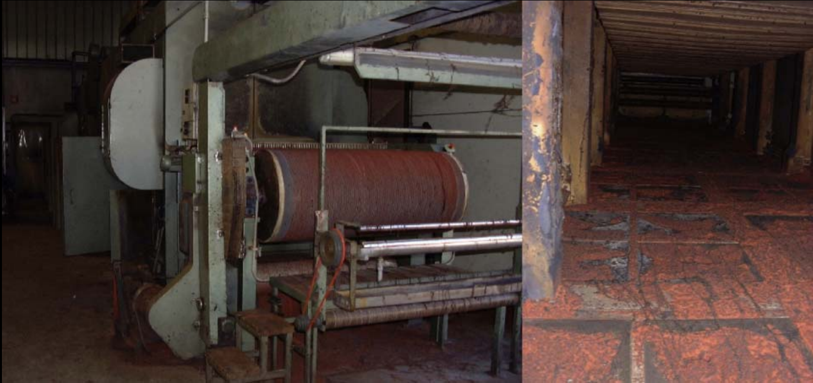
Inlet section of a nylon flocking machine
